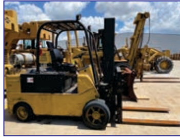
12,000 Lb. TowMotor Model 670S Forklift, 146" Lift Height, 24" Load Center, 3143 Hours on Meter
