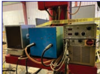
Clad Unit #3: A&N Plant Model RC4X3.75 Cladding Machine (S/N 2917), Arc Specialties Hot One Solid State Hotwire Power Supply (S/N 1161-20329), 122" boom vert. trvl, 69" hor. trvl, 218" overall ht., Esab 350 MPI MIG Welder, Best Welds Welding Torch Water Cooler (S/N LJ430006F)
