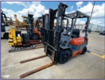
5,000 Lb. Toyota Model 42-GF025 Forklift, 131.5" Lift Height, 20" Load Center, 10 deg. Back Tilt, Side Shift, 8991 Hours on Meter
