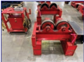
5 Ton Weldwire WWRT 10 Turning Rolls
