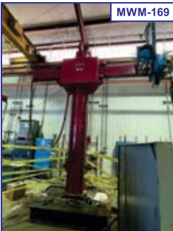
Clad Unit #3: A&N Plant Model RC4X3.75 Cladding Machine (S/N 2917), Arc Specialties Hot One Solid State Hotwire Power Supply (S/N 1161-20329), 122" boom vert. trvl, 69" hor. trvl, 218" overall ht., Esab 350 MPI MIG Welder, Best Welds Welding Torch Water Cooler (S/N LJ430006F)
