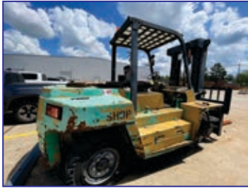
11,000 Lb. Dalian (Vanguard) Model CPCD50 Forklift, 118" Lift height, 24" Load Center, 20 IPS Lift Speed, 16 MPH Travel Speed
