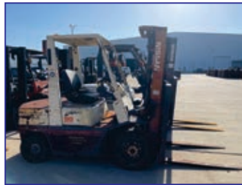
4,300 Lb. Nissan Model KPH02A25V (50 Enduro) Forklift, 187" Lift Height, 24" Load Center, 3F475 Mast, Forks, Gas Powered, 2149 Hours on Meter
