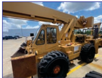
15 Ton Dresser Dressta Model 150FA Rough Terrain Crane, 17.5' Min. Ht. at Max. Raise Angle, 37.5' Max. Ht. at Max. Raise Angle (no jib), 70° Max. Elev., 8.67' Max. Tail Swing, 108 HP, 20.2 MPH Forward Speed, 11.1 MPH Reverse, Outriggers, S/N 10062
