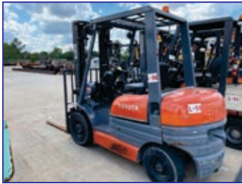
5,000 Lb. Toyota Model 42-GF025 Forklift, 131.5" Lift Height, 20" Load Center, 10 deg. Back Tilt, Side Shift, 8991 Hours on Meter
