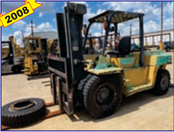
11,000 Lb. Dalian (Vanguard) Model CPCD50 Forklift, 118" Lift height, 24" Load Center, 20 IPS Lift Speed, 16 MPH Travel Speed
