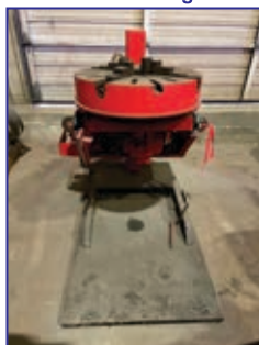
26" Tilt/Turn Positioner w/ 25" 4-Jaw Chuck
