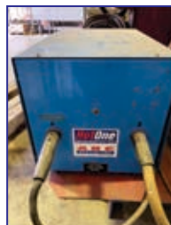
Clad Unit #5: Vanguard LHZ34 Automatic Cladding Machine, Arc Specialties Hot One Solid State Hotwire Power Supply, 118" boom vert. trvl, 175.5" boom hor. trvl, +/-180° col. rot., Esab MTS-3500i MIG Welder, EST Welds Welding Torch Water Cooler
