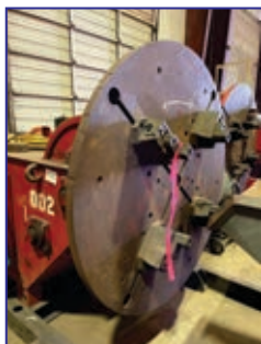
60" Tilt/Turn Welding Positioner w/ 4 HD Jaws
