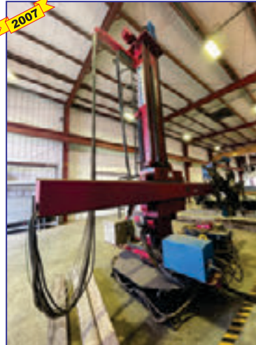
Clad Unit #5: Vanguard LHZ34 Cladding Machine with Arc Specialties Hot One Solid State Hotwire Power Supply Esab MTS-3500i MIG Welder, Note: (2) rotary tables avail.
