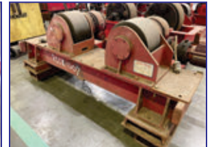
20 Ton Vanguard HGK-20 Turning Rolls
