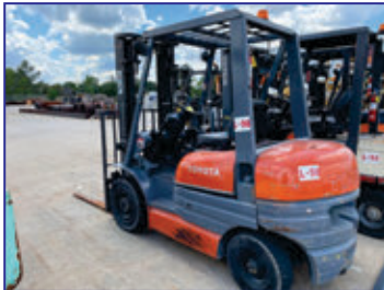
5,000 Lb. Toyota Model 42-GF025 Forklift, 131.5" Lift Height, 20" Load Center, 10 deg. Back Tilt, Side Shift, 8991 Hours on Meter
