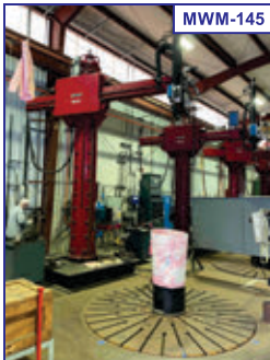
Clad Unit #1: A&N Plant Model RC40X3.75 Cladding Machine S/N 3160/3202), Arc Specialties Hot One Solid State Hotwire Power Supply (S/N 1018-20031), 100" dia. table, 118" mm boom vert. trvl, 69" boom hor. trvl, 213" overall ht., Thermal Arc DC TIG Arc Starter, Esab 350 MPI MIG Welder (S/N WE-J045029), Bernard 3500SS TIG/MIG Welding Torch Water Cooler
