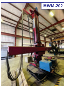
Clad Unit #5: Vanguard LHZ34 Automatic Cladding Machine, Arc Specialties Hot One Solid State Hotwire Power Supply, 118" boom vert. trvl, 175.5" boom hor. trvl, +/-180° col. rot., Esab MTS-3500i MIG Welder, EST Welds Welding Torch Water Cooler
