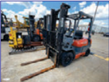
5,000 Lb. Toyota Model 42-GF025 Forklift, 131.5" Lift Height, 20" Load Center, 10 deg. Back Tilt, Side Shift, 8991 Hours on Meter
