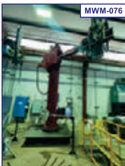
Clad Unit #4: A&N Plant Model RC4X3.75 Cladding Machine (S/N 2558), Arc Specialties Hot One Solid State Hotwire Power Supply (S/N 0999-96006), 100" dia. table, 122" boom vert. trvl, 69" hor. trvl, 218" overall ht., Esab 350 MPI MIG Welder, DC TIG Arc Starter, Best Welds Welding Torch Water Cooler
