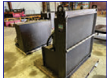
MTS Model 510.230 Hydraulic Power System with Young Oil Cooler
