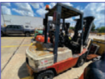
3,700 Lb. Nissan Model PJ02A20V Forklift, 187" Lift Height, 24" Load Center, 3F475 mast, single fork, 69,302 Hours on Meter
