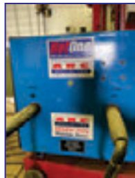
Clad Unit #2: A&N Plant Model RC40X3.75 Cladding Machine (S/N 3163), Arc Specialties Hot One Solid State Hotwire Power Supply (S/N 1216-20436), 100" dia. table, 118" mm boom vert. trvl, 69" boom hor. trvl, 213" overall ht., Esab X Series MTS-3500i Welder (S/N MORJ833003)
