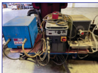
Clad Unit #5: Vanguard LHZ34 Automatic Cladding Machine, Arc Specialties Hot One Solid State Hotwire Power Supply, 118" boom vert. trvl, 175.5" boom hor. trvl, +/-180° col. rot., Esab MTS-3500i MIG Welder, EST Welds Welding Torch Water Cooler
