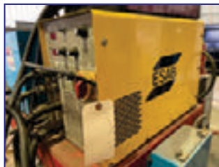
Clad Unit #1: A&N Plant Model RC40X3.75 Cladding Machine with Arc Specialties Hot One Solid State Hotwire Power Supply and Esab 350 MPI MIG Welder
