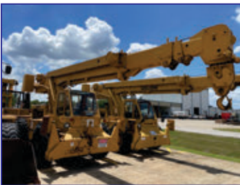
15 Ton Dresser Dressta Model 150FA Rough Terrain Crane, 17.5' Min. Ht. at Max. Raise Angle, 37.5' Max. Ht. at Max. Raise Angle (no jib), 70° Max. Elev., 8.67' Max. Tail Swing, 108 HP, 20.2 MPH Forward Speed, 11.1 MPH Reverse, Outriggers, S/N 10062
