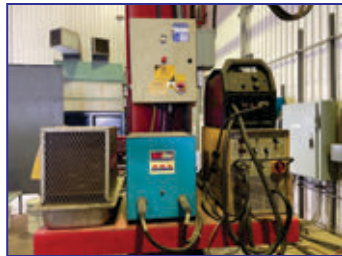
Clad Unit #1: A&N Plant Model RC40X3.75 Cladding Machine S/N 3160/3202), Arc Specialties Hot One Solid State Hotwire Power Supply (S/N 1018-20031), 100" dia. table, 118" mm boom vert. trvl, 69" boom hor. trvl, 213" overall ht., Thermal Arc DC TIG Arc Starter, Esab 350 MPI MIG Welder (S/N WE-J045029), Bernard 3500SS TIG/MIG Welding Torch Water Cooler
