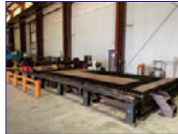
Plasma Systems Model 2010H Plasma Table, 264" x 118" Table, Burny 10 LCD
