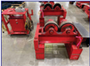
5 Ton Weldwire WWRT 10 Turning Rolls
