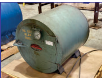
Phoenix Model 1.5B Dry Rod Electrode Stabilizing Oven, S/N 15B-1
