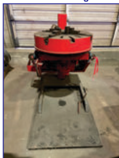
26" Tilt/Turn Positioner w/ 25" 4-Jaw Chuck
