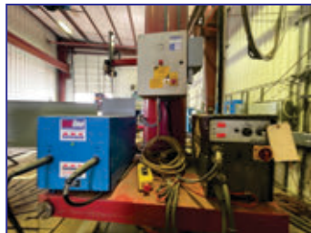
Clad Unit #2: A&N Plant Model RC40X3.75 Cladding Machine (S/N 3163), Arc Specialties Hot One Solid State Hotwire Power Supply (S/N 1216-20436), 100" dia. table, 118" mm boom vert. trvl, 69" boom hor. trvl, 213" overall ht., Esab X Series MTS-3500i Welder (S/N MORJ833003)
