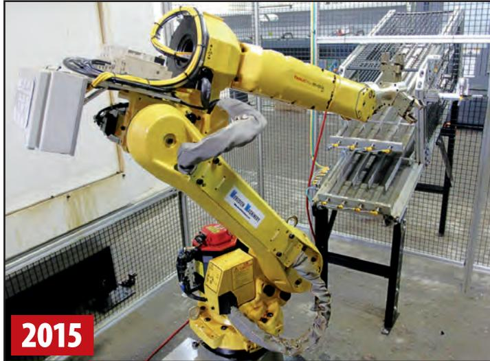
FANUC M-10IA/12 6-AXIS CNC ROBOT
