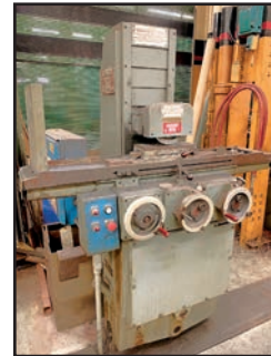
BROWN & SHARPE 618 MICROMASTER SURFACE GRINDER
