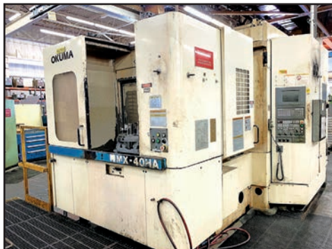
OKUMA MX-40HA CNC HORIZONTAL MACHINING CENTER
