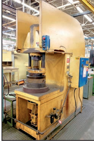
100-TON HANNIFIN HYDRAULIC PRESS
