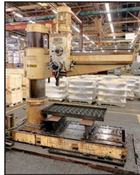
Ooya RE2-1450D 5' X 13" RADIAL ARM DRILL
