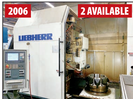
LIEBHERR LFS-800 CNC GEAR SHAPER
