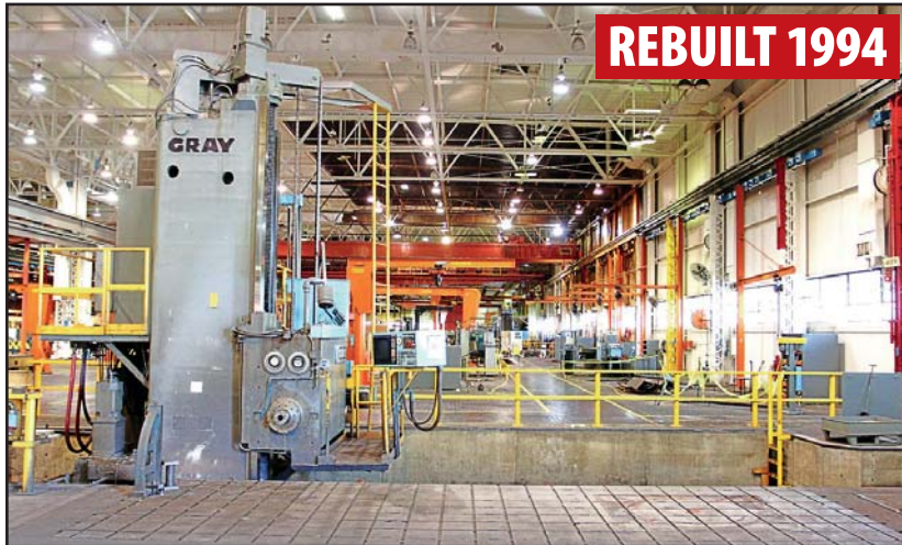
GRAY 6" FLOOR-TYPE HORIZONTAL BORING MILL
