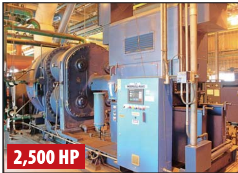
2,500 HP INGERSOLL RAND CENTAC CENTRIFUGAL AIR COMPRESSOR
