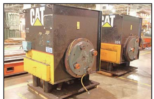
7,800-LB. ARONSON HS6GF/TS6GE HEADSTOCK/ TAILSTOCK WELDING POSITIONERS
