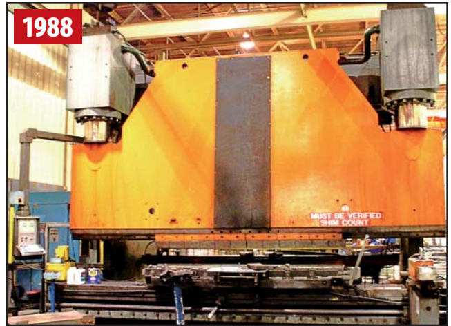
1,100-TON LVD BH20 CNC HYDRAULIC BRAKE
