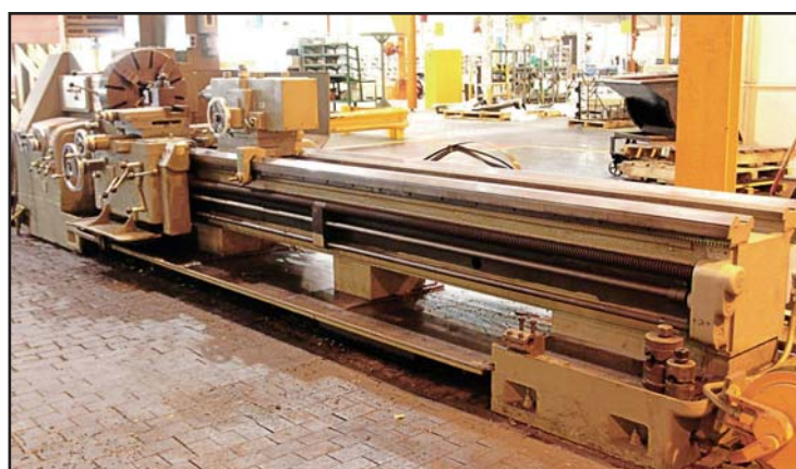
AMERICAN 20" X 144" STYLE E ENGINE LATHE
