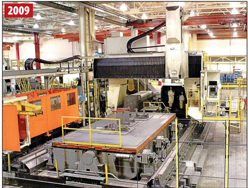
MAG CINCINNATI U5 4 METER 5-AXIS CNC GANTRY MILL
