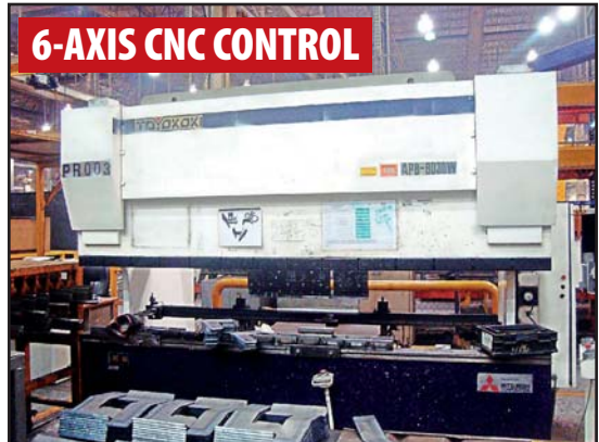
88-TON TOYOKOKI APB-8030W 6-AXIS CNC PRESS BRAKE
