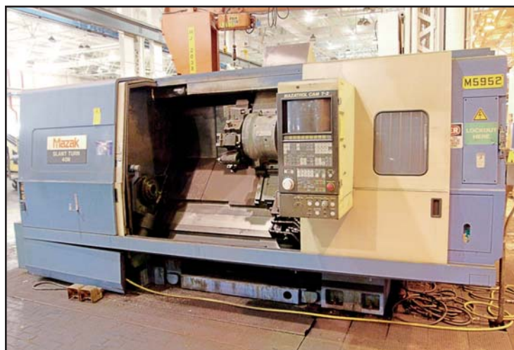
MAZAK SLANT TURN 40N SLANT BED LATHE
