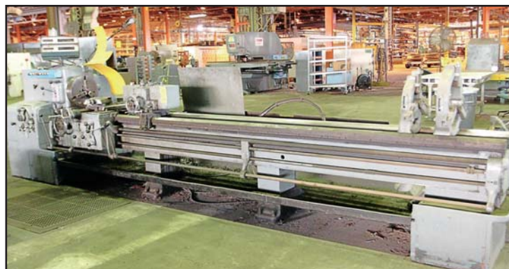
AMERICAN 14" X 150" STYLE B ENGINE LATHE
