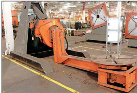
IRCO I-24 BEAM TYPE WELDING POSITIONER
