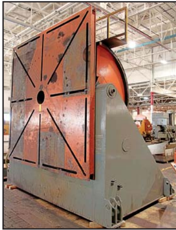
< 120,000-LB. ARONSON G1200CS TILT/TURN WELDING POSITIONER
