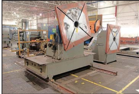
25,000-LB. ARONSON HS25/TS25 HEADSTOCK TAILSTOCK WELDING POSITIONERS
