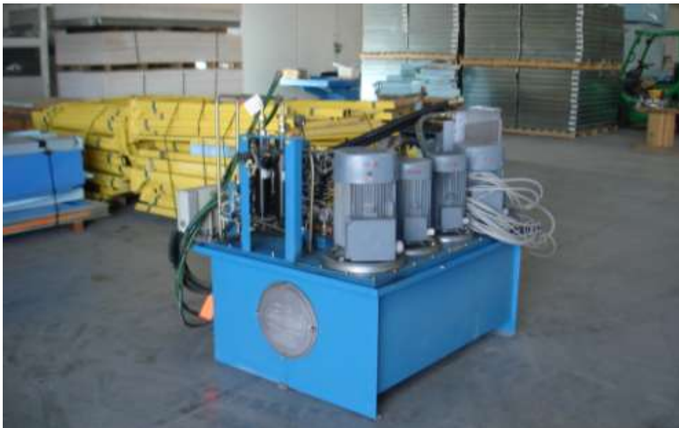
Figure 23: Press and Scissor Lift Hydraulic Pump System
