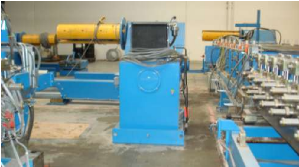
Figure 22: Hydraulic pump for roll formers
