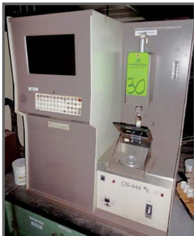
LECO CORPORATION CS-444 CARBON/SULFUR DETERMINATOR
