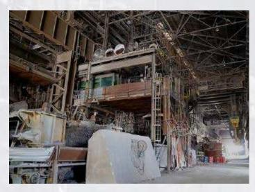
4,722 tons/day; 1,666,866 tons/year; 180 ton ladle capacity LMF; Ladle in car design, 32- MVA reheating transformer, Argon stirring, belt feed alloy additive system; 18" diameter electrode, 3 ladle transfer cars, Emission control system, cooling water, degassing, chemistry lab, computer controls; 165 ton charging ladle, total shell weight 55,000lb; 150 ton hot metal ladles, enlarged to 175 ton in 1994; 170 ton teaming ladles
