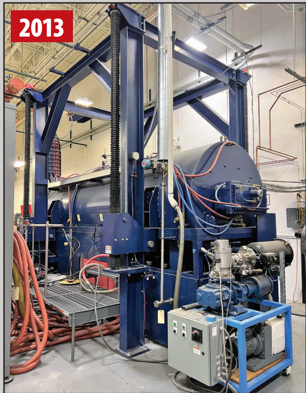
CENTORR VACUUM INDUSTRIES "LARGE AREA NET-SHAPE CRYSTAL EXTRACTION" GROWTH FURNACE
