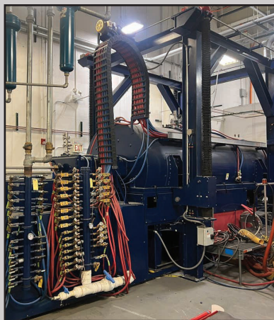
CENTORR VACUUM INDUSTRIES "LARGE AREA NET-SHAPE CRYSTAL EXTRACTION" GROWTH FURNACE
