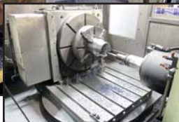
KURAKI KBM-11A 5-AXIS CNC HORIZONTAL BORING MILL
