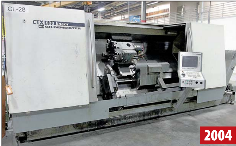
GILDEMEISTER CTX 620 LINEAR 6-AXIS CNC MILL/TURN CENTER
