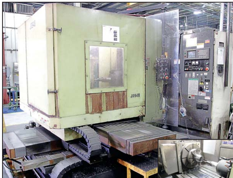
KURAKI KBM-11A 5-AXIS CNC HORIZONTAL BORING MILL
