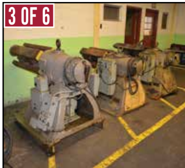
(6) LITTELL No. 60 Coil Reels to 15,000-lb. Capacity
