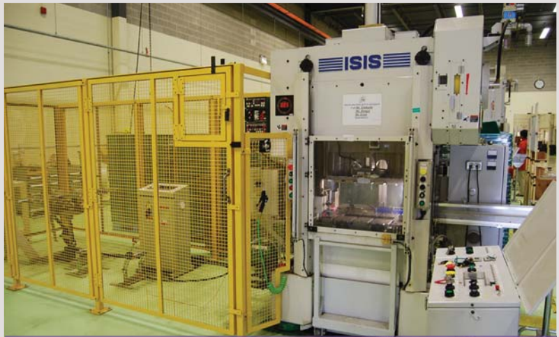
44 Ton ISIS 40SH Straight Side High Speed Mechanical Stamping Press, s/n 290 (2006)
