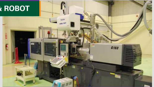
83 Ton Sumitomo SE75DU Direct-Drive Electric Horizontal Injection Molder, s/n M0SG5021 (2006)
