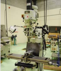
First LC-11/2VS Vertical Milling Machine, s/n 41028942
