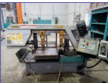
Hyd-Mech S-23P Horizontal Bandsaw, 16" x 20" cap., mitering, 75-350 fpm, 8.8 hp motor, coolant
