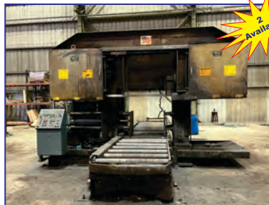
HEM DC-4040 Horizontal Bandsaw, new 1994, 40" x 40" cap., 2-5/8" blade, coolant, power feed
