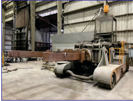
20,000 Lb. Dango Trackless Manipulator , 126" width, 144" whl base, 228" length, 108" reach, 60" max. tong ht., 60" max. tong opening, updated electronics
