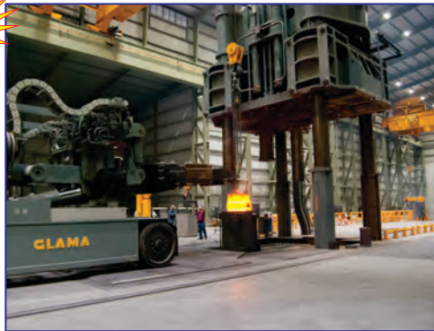
Forging Cell with 6500 Ton and 3300 Ton Presses
