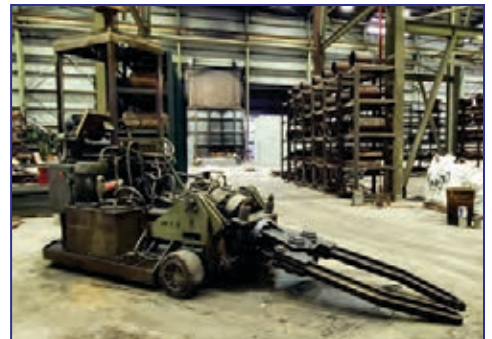
3,000 Lb. Glama Trackless Manipulator , 84" width, 96" whl base, 144" length (w/o tongs), 96" tong length, 96" reach, 72" lift ht.
