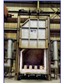
W11, 1850 Deg. F, 98" W x 68" H x 82" D, natural gas, 2 burners, fiber lined, Honeywell controls
