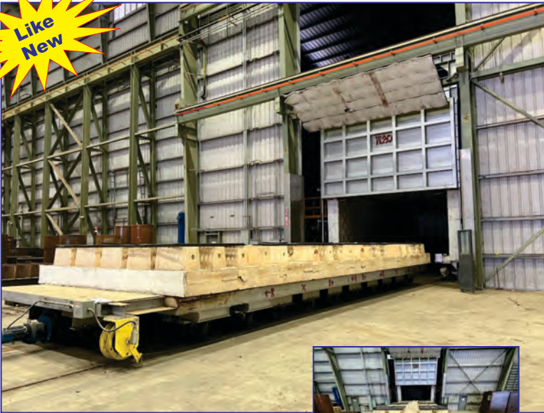
W20, 1850 Deg. F Epcon Car Bottom Furnace, 193" W x 115" H x 481" D, natural gas fired, 20 burners, 5 zones, fiber lined, Honeywell controls with PLC
