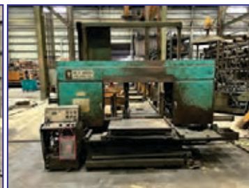
W.F Wells Horizontal Bandsaw, 32" x 24" cap., 2" blade, chip conv.
