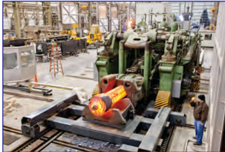
120,000 Lb. DEMAG MEER Track Bound Manipulator with hot forging billet
