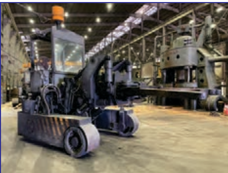
8,000 Lb. Glama Trackless Manipulator , 100" width, 98" whl base, 132" length (w/o tongs), 96" tong length, 96" reach, 72" max. tong ht., 62" max. tong opening
