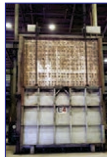
E4, 2100 Deg. F North American Mfg. Furnace, 170" W x 117" H x 140" D, natural gas, 6 burners, fiber lined, Honeywell controls
