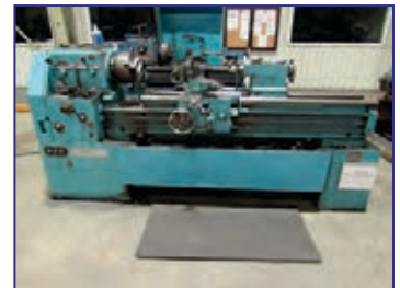
16" x 60" Summit Gap Bed Engine Lathe , 16" swing, 22" in gap, 60" ctrs, 3-jaw chuck, 1500 rpm, Aloris tool holder, tailstock, taper attach.,
