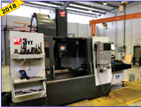
Haas VF-3YT CNC VMC, new 2018 , 24" x 54" table, 50 taper, 10,000 rpm, 30 hp, 40" X / 26" Y / 25" Z, 7.9" - 32.9" spindle nose to table, 30 tool ATC, Midaco pallet changer
