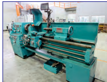
18" x 66" Andrychow Gap Bed Engine Lathe , 18" swing, 11" over slide, 23" in gap, 66" ctrs, 2" hole, DRO, Aloris, 10" 3-jaw chuck, tailstock, taper attach., coolant
