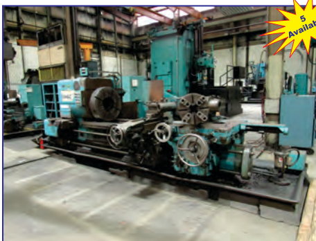
Gisholt 4L Turret Lathes , 24" to 28" 4-jaw chucks, 9.75" to 12.5" thru-holes, 60" to 96" bed lengths, hex tool turrets
