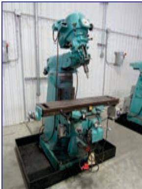
Alliant Vertical Mill , 9" x 47" table, 60-4500 rpm, 2 hp, DRO, pwr cross feed, pwr in/out feed
