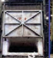
F6, 2200 Deg. F, 160" W x 118" H x 106" D, natural gas, 4 burners, fiber lined, Honeywell controls
