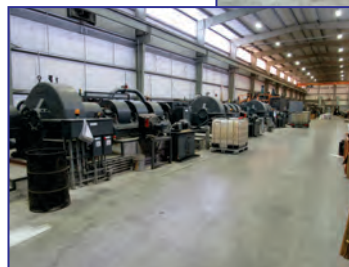
2500 Ton Babcock & Wilcox Preforming Press, 32" x 157" Bed with 57" Travel, 35" x 63" Sliding Ram with 8" Travel, 114" Daylight, 52" Stroke, 76" Btwn Uprights, 42" Window Width, FSI PLC Controlled
