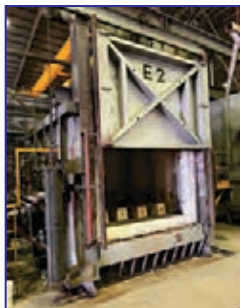
E2, 2100 Deg. F, 94" W x 65" H x 108" D, natural gas, 4 burners, fiber lined, Honeywell controls
