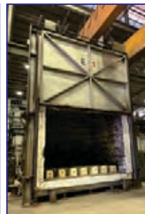
E5, 2100 Deg. F, 165" W x 118" H x 140" D, natural gas, 6 burners, fiber lined, Honeywell controls
