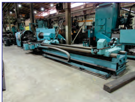
VDF Wohlenberg Type E1120 Lathe , 46" swing, 32" over slide, 39" face plate w/ 4 jaws, 3" hole, 276" ctrs, 315 rpm, roller steady, chuck on tailstock, motorized tailstock
