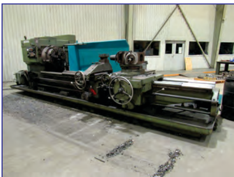
Warner & Swasey 5A Turret Lathe , 144" chuck to turret, 28" 4-jaw chuck, 12.5" hole, 75 hp, 4-pos. front toolpost, rear hex turret, rapids, coolant
