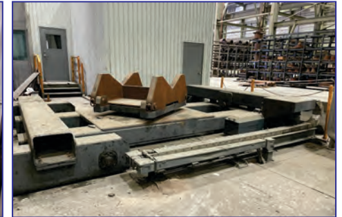
Billet Rail Car , 120" rail span, rotating platform 24" above floor, hyd. rotation and cart traverse, three speed selection, push button controls
