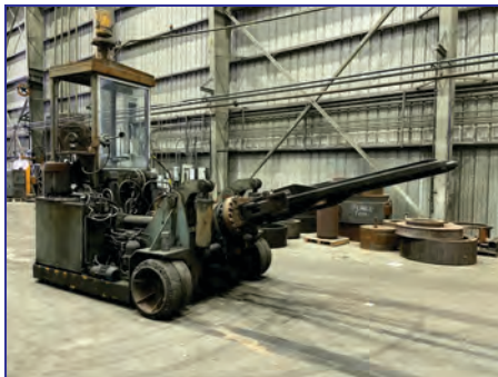
3,000 Lb. Glama Trackless Manipulator , 84" width, 96" whl base, 144" length (w/o tongs), 96" tong length, 96" reach, 72" lift ht.
