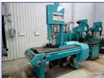
Marvel Series 8 Mark II Vertical Bandsaw, 18" x 22" cap., 50-450 fpm, 5 hp motor, mitering, coolant
