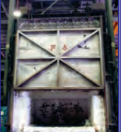
F3, 2200 Deg. F, 160" W x 118" H x 106" D, natural gas, 4 burners, fiber lined, Honeywell controls
