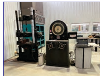
Southwark-Emery Compression Tester , 120,000 lbs. comp. cap., 34" max. part length
