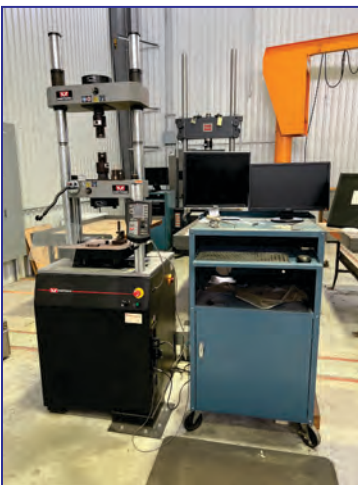
Intron Type UTM-HYD Model 300DX-C3A-G1E Industrial Tension, Compression, and Shear Testing Machine , 67,500 lb.-ft. load cap., 6 IPM test speed, 6" actuator stroke, 36" tension opening, 96" max. oper. ht., 10.6" - 42" specimen lengths
