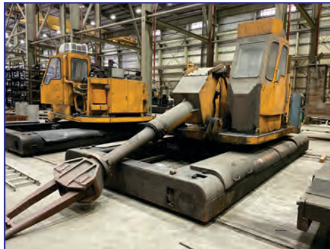
3,000 Lb. Columbiana Rail Bound Manipulator , 216" rail span, 242" width, 96" btwn axles, 120" length, 17 ft. reach from rotation ctr, 12 ft. max. ext. reach, 108" trvl in/out, 72" max. tong ht., updated electronics
