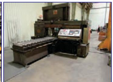
HEM CT2000HA-DC-C Horizontal Bandsaw, 20" x 20" cap., 48" stroke shuttle vise, 20 hp, (2) 120" powered conveyors, bundling, chip auger, coolant
