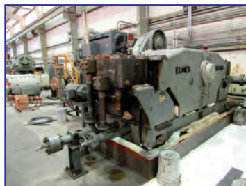
2500 Ton Babcock & Wilcox Preforming Press, 32" x 157" Bed with 57" Travel, 35" x 63" Sliding Ram with 8" Travel, 114" Daylight, 52" Stroke, 76" Btwn Uprights, 42" Window Width, FSI PLC Controlled
