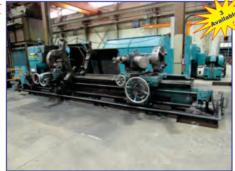
Gisholt 5L Longbed Turret Lathes , 32" 4-jaw chucks, 9.75" to 12.75" thru-holes, 120" to 144" bed lengths, hex turrets
