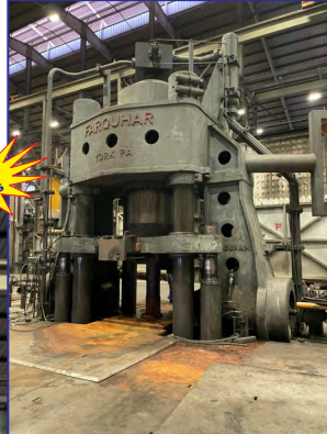
2014, Babcock & Wilcox 6500 Ton Open Die Forging Press, 90" x 290" Sliding Bed with 168" of Trvl, 136" x 300" Ram with 80" of Trvl, 240" Daylight, 120" Stroke, 144" Between Uprights, 160" Wide Windows, FSI PLC Controlled
