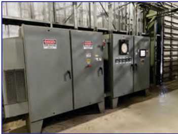
W20, 1850 Deg. F Epcon Car Bottom Furnace, 193" W x 115" H x 481" D, natural gas fired, 20 burners, 5 zones, fiber lined, Honeywell controls with PLC
