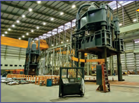
6500 / 3300 Ton Open Die Forging Cell, Overall view (above) and partial view of Central Control System (below)
