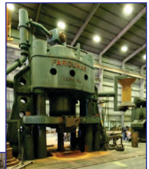
2014, Babcock & Wilcox 3300 Ton Open Die Forging Press, 84" x 210" Sliding Bed with 116" of Trvl, 42" x 88" Ram, 240" Daylight, 120" Stroke, 54" Between Uprights, 112" Window Width
