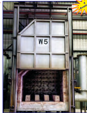
W5 / W6 / W7 / W8, 1850 Deg. F, 97" W x 58" H x 86" D, natural gas, 2 burners, fiber lined, Honeywell controls
