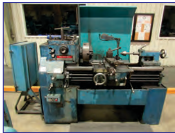
16" x 36" LeBlond Engine Lathe , 16" swing, 36" ctrs, 12" 3-jaw chuck Aloris tool holder, tailstock, taper attach., work light
