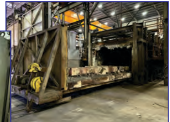
(above/left) E6, 2400 Deg. F Custom Built Car Bottom Furnace, 135" W x 80" H x 320" D, natural gas fired, 14 burners, fiber lined, Honeywell controls
