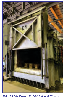
E1, 2100 Deg. F, 98" W x 62" H x 108" D, natural gas, 4 burners, fiber/brick lined, Honeywell controls
