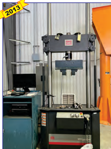
MTS 370.50 Fatigue Tester, new 2013, 500 kN force, 6" actuator stroke, 13" - 78" specimen length
