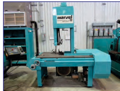
Marvel Series 8 Mark II Vertical Bandsaw, 18" x 22" cap., 50-450 fpm, 5 hp motor, mitering, coolant
