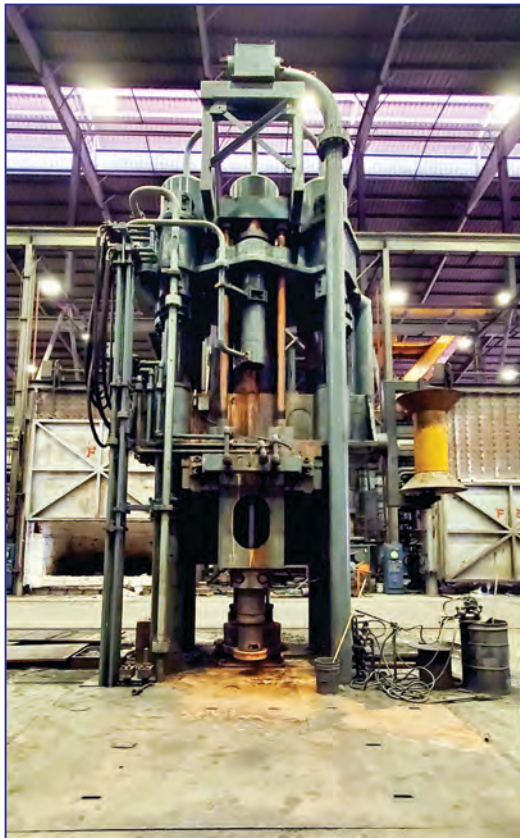
2500 Ton Babcock & Wilcox Preforming Press, 32" x 157" Bed with 57" Travel, 35" x 63" Sliding Ram with 8" Travel, 114" Daylight, 52" Stroke, 76" Btwn Uprights, 42" Window Width, FSI PLC Controlled
