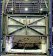
F4, 2200 Deg. F, 160" W x 80" H x 108" D, natural gas, 4 burners, fiber lined, Honeywell controls
