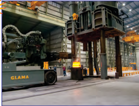
Forging Cell with 6500 Ton and 3300 Ton Presses
