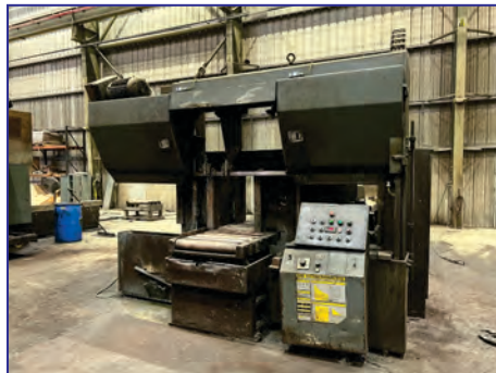
Hyd-Mech H-22A Horizontal Bandsaw, 24" x 24" cap., bundle attach., power feed
