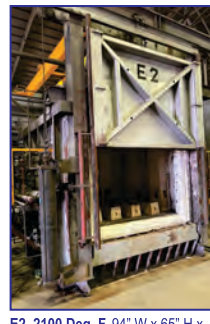
E2, 2100 Deg. F, 94" W x 65" H x 108" D, natural gas, 4 burners, fiber lined, Honeywell controls
