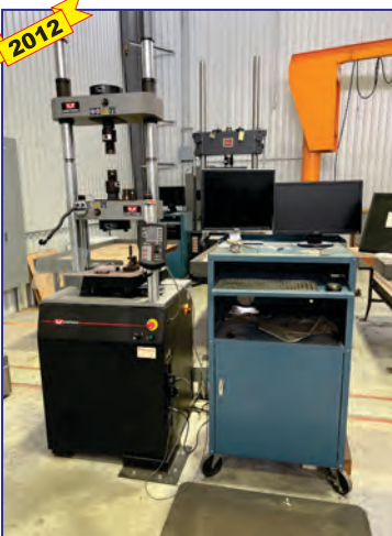
Instron Type UTM-HYD Model 300DX-C3A-G1E Industrial Tension, Compression, and Shear Testing Machine, new 2012, 67,500 lb.-ft. load cap., 6 IPM test speed, 6" actuator stroke, 36" tension opening, 96" max. oper. ht., 10.6" - 42" specimen lengths
