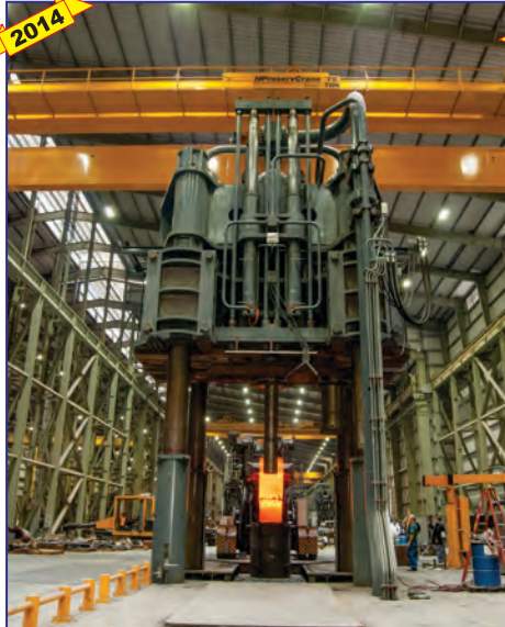
2014, Babcock & Wilcox 6500 Ton Open Die Forging Press, 90" x 290" Sliding Bed with 168" of Trvl, 136" x 300" Ram with 80" of Trvl, 240" Daylight, 120" Stroke, 144" Between Uprights, 160" Wide Windows, FSI PLC Controlled
