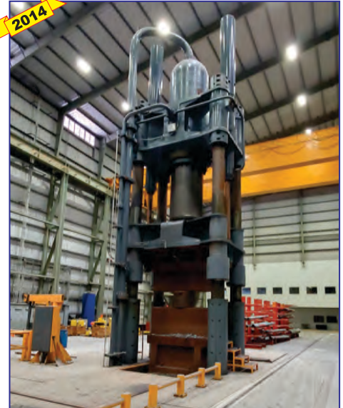
2014, Babcock & Wilcox 3300 Ton Open Die Forging Press, 84" x 210" Sliding Bed with 116" of Trvl, 42" x 88" Ram, 240" Daylight, 120" Stroke, 54" Between Uprights, 112" Window Width
