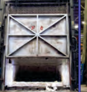
F6, 2200 Deg. F, 160" W x 118" H x 106" D, natural gas, 4 burners, fiber lined, Honeywell controls
