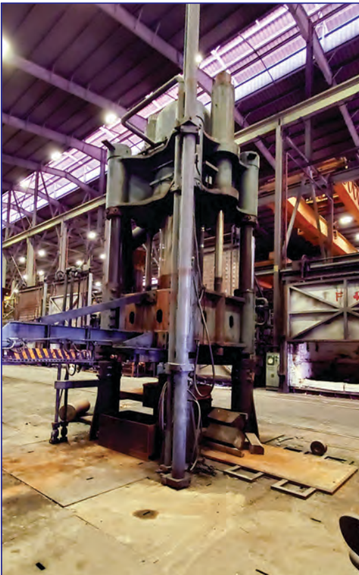
1400 Ton Lake Erie Press, 40" x 135" Bed with 96" Stroke, 36" x 93" (2) Station Die with 48" of Travel, 120", Daylight, 62" Stroke, 58" Btwn Uprights, 57" Window Width
