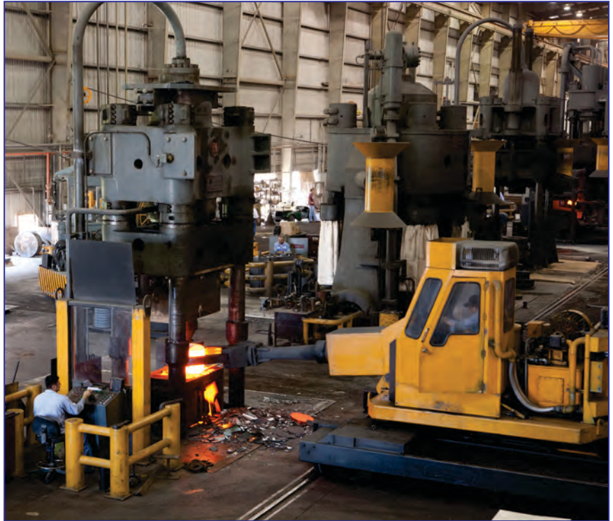
HPM 1000 Ton Forging Press, 48" x 66" Bed, 48" x 67" Ram, 98" Daylight, 34" Stroke, 69" Between Uprights
