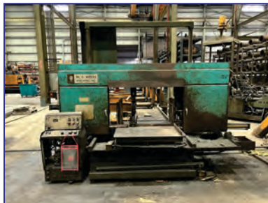
W.F. Wells Horizontal Bandsaw, 32" x 24" cap., 2" blade, chip conv.
