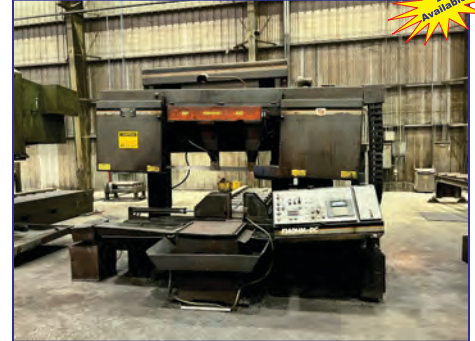
HEM F140HM-DC Horizontal Bandsaw, new 2000, 24" x 22" cap., 20 hp, chip auger, coolant, power infeed
