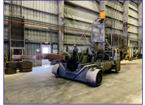
16,000 Lb. Salem Trackless Manipulator , 120" width, 120" whl base, 200" length (w/o tongs), 84" tong length, 96" reach, 78" max. tong ht., 62" max. tong opening
