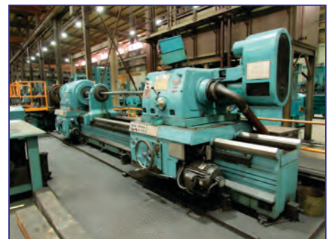
VDF Wohlenberg Model B10SP Deep Hole Gun Drill , 196" stroke, 8" hole, 60 hp, 895 rpm, 136" x 36" cross sliding table, DRO on drill and table, coolant system w/ chiller
