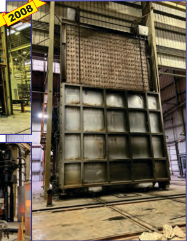
(above/left) East Side, 2500 Deg. F Custom Built Car Bottom Furnace, 216" W x 180" H x 300" D, natural gas fired, 10 burners, 2 zones, fiber lined, Honeywell controls with PLC
