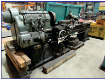
20" x 72" Monarch Engine Lathe , 20" swing, 72" ctrs, 15" 4-jaw chuck, 6" steady rest, tailstock, taper attach.
