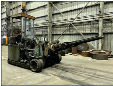
3,000 Lb. Glama Trackless Manipulator , 84" width, 96" whl base, 144" length (w/o tongs), 96" tong length, 96" reach, 72" lift ht.
