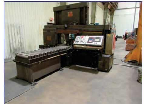
HEM CT2000HA-DC-C Horizontal Bandsaw, 20" x 20" cap., 48" stroke shuttle vise, 20 hp, (2) 120" powered conveyors, bundling, chip auger, coolant
