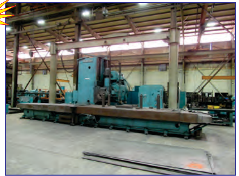
Ingersoll Horizontal Milling Machine , 48" x 192" table, 144" cross trvl, 60" vert. trvl, 18" quill trvl, 60 taper, 100 hp (est.)
