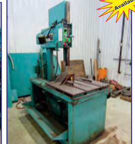
Metal Mizer Model MS2018-2 Vertical Bandsaw, 18" x 18" cap., 99-275 fpm, 2 hp motor, mitering
