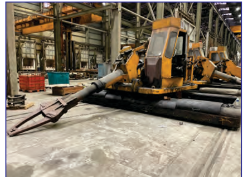
3,000 Lb. Hopkins Kendall Rail Bound Manipulator , 216" rail span, 242" width, 96" btwn axles, 120" length, 17 ft. reach from rotation ctr, 12 ft. max. ext. reach, 108" trvl in/out, 72" max. tong ht., updated electronics
