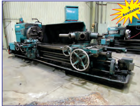
Gisholt 5L Turret Lathes , 28" to 32" 4-jaw chucks, 9.75" to 12.75" thru-holes, 84" to 96" bed lengths, hex tool turrets
