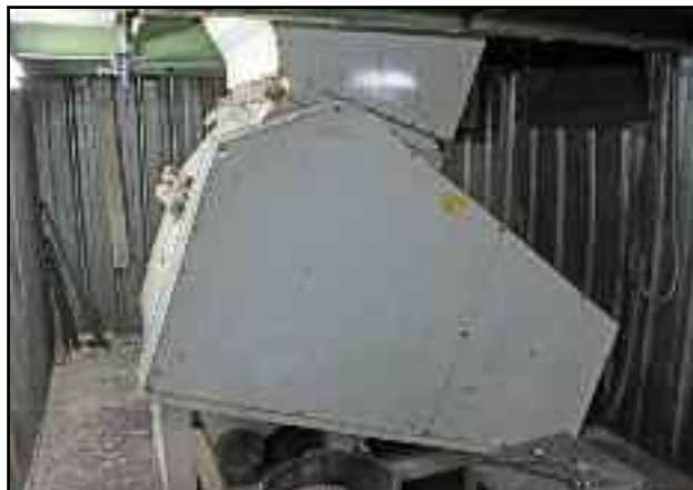
• (2) Mecanofil Type 70/98 Granulators (2004) Main Motor 112.5 HP/75 kW, Opening 400 mm x 965 mm
