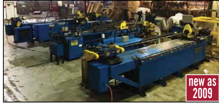
(3) HORN (HMT) 2RCNC & 2LCNC 2" and EATON LEONARD VB30 3" Hydraulic CNC Tube Benders
