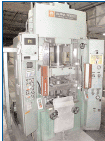
ALPHA PRESS 128D/9-20, 125-TON HYDRAULIC POWDER COMPACTING PRESS
