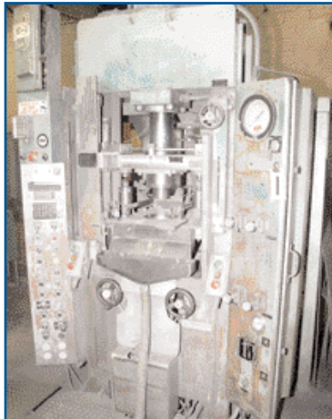
ALPHA PRESS APC-64D-15L, 60-TON HYDRAULIC POWDER COMPACTING PRESS
