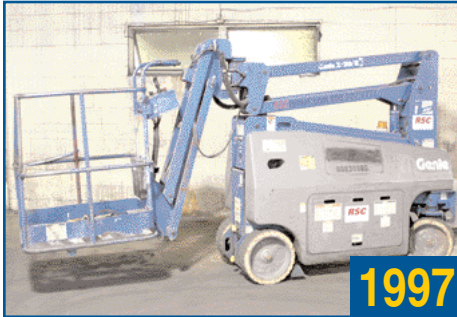
1997 GENIE MODEL Z-20/8N NARROW AISLE ARTICULATED BOOM ELECTRIC PERSONNEL LIFT
