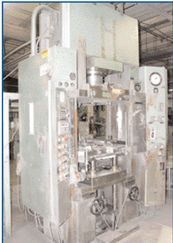
ALPHA PRESS 253D-16L, 250-TON HYDRAULIC POWDER COMPACTING PRESS
