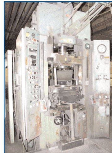
ALPHA PRESS 128D-16L, 125-TON HYDRAULIC POWDER COMPACTING PRESS
