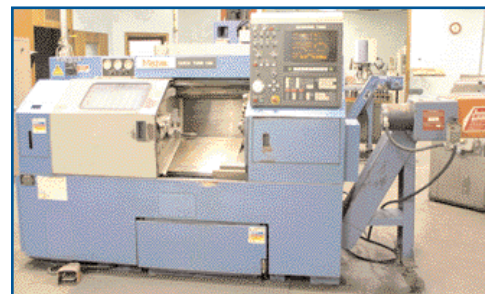
MAZAK MODEL QT-15-N-UNIV-K 2-AXIS CNC TURNING CENTER
