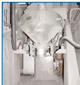
PATTERSON INDUSTRIES TYPE "A" THORO-BLENDER POWDER BLENDER/MIXER
