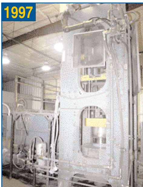
500-TON, BEST PRESS 500-TON POWDER COMPACTING PRESS
