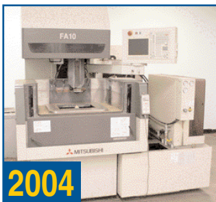
2004 MITSUBISHI MODEL FA10M 5-AXIS CNC WIRE CUT EDM
