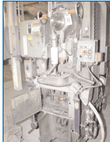
STOKES PENNWALT MODEL 900-526-1 (NEWER VERSION OF MODEL R-4), 20-TON MECHANICAL POWDER COMPACTING PRESS
