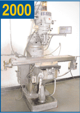
SHARP MODEL LMV-50 3-HP VARIABLE SPEED VERTICAL MILLING MACHINE
