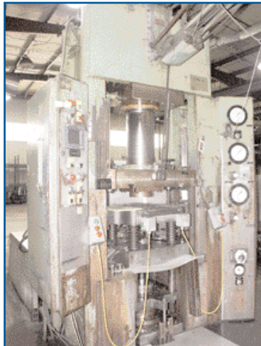
250-TON, ALPHA PRESS MODEL APC-250/2 250-TON HYDRAULIC PRESS
