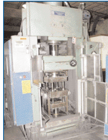
220-TON, MANNESMANN (POWDER-MATE) MODEL HPM-220, 220-TON HYDRAULIC POWDER COMPACTING PRESS
