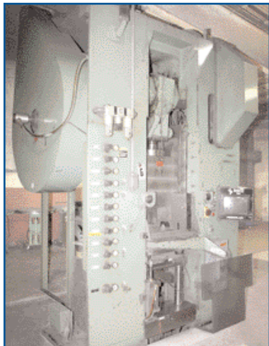
GASBARRE 200-STD, 200-TON STRAIGHT SIDE MECHANICAL POWDER COMPACTING PRESS
