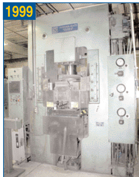
DIGITAL PRESS POWDER-MATE MODEL PM-250, 250-TON HYDRAULIC POWDER COMPACTING PRESS
