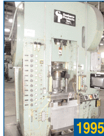
GASBARRE 200 UP SIZER 200-TON STRAIGHT SIDE MECHANICAL UPRIGHT SIZING PRESS
