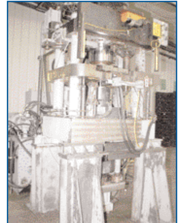
MULTIPRESS 400-TON 4-POST VERTICAL DOUBLE-ACTING HYDRAULIC PRESS
