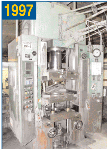
ALPHA PRESS 253D/3-18, 250-TON HYDRAULIC POWDER COMPACTING PRESS
