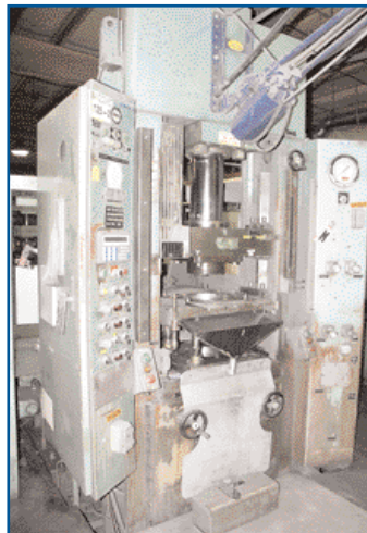
ALPHA PRESS 128D-16L, 125-TON HYDRAULIC POWDER COMPACTING PRESS
