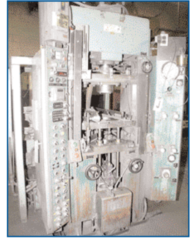
ALPHA PRESS APC-64D-14L, 60-TON HYDRAULIC POWDER COMPACTING PRESS
