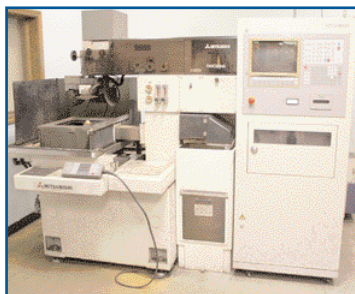
MITSUBISHI MODEL DWC-90HA 4-AXIS CNC WIRE CUT EDM
