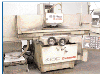
OKAMOTO MODEL ACC-1224-DX 12" X 24" HYDRAULIC SURFACE GRINDER
