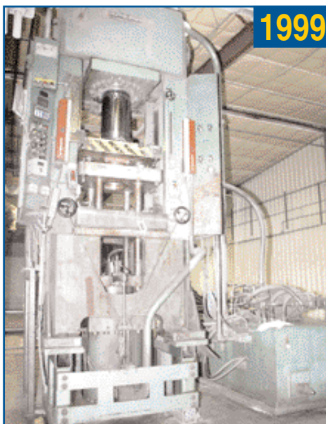
ALPHA PRESS MODEL 755D/9-20, 750-TON HYDRAULIC POWDER COMPACTING PRESS
