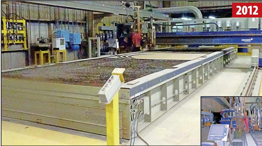
MESSER MPC2016 (3)-HEAD CNC PLASMA CUTTING SYSTEM
