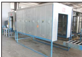
CATALYTIC INDUSTRIAL SYSTEMS INFRARED PASS-THROUGH OVEN
