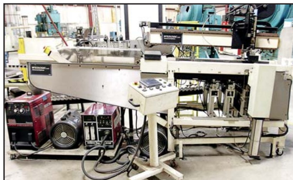
WELD LOGIC SEAM WELDER CELL INCL. SHEET METAL ROLLER
