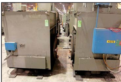
32,000 LB CAPACITY ARONSON HS16GE TS16GE HEADSTOCK TAILSTOCK WELDING POSITIONER SET
