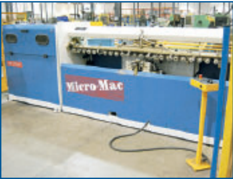
PAVE TRUELINE MODEL MICRO-MAC 3D CNC WIRE FORMING MACHINE
