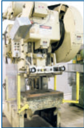
60 TON MINSTER MODEL NO. 6 O.B.I MECHANICAL PRESS
