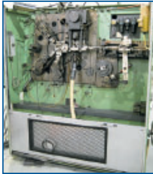
BIHLER MODEL MACH 1/7 WIRE FORMING MACHINE
