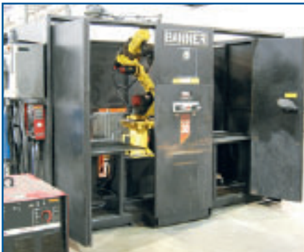
BANNER LINCOLN ELECTRIC AUTOMATION SYSTEM 30 (2) STATION ROBOTIC WELDING CELL
