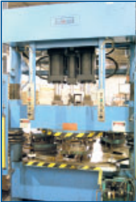
BECKWOOD MODEL 10058 TWO POST, TRIPLE RAM, HYDRAULIC PRESS
