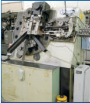
BIHLER MODEL RM-35 WIRE FORMING MACHINE
