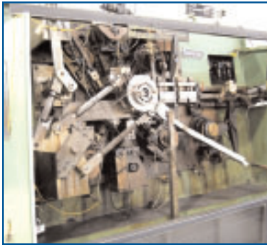
BIHLER MODEL GRM-80 WIRE FORMING MACHINE
