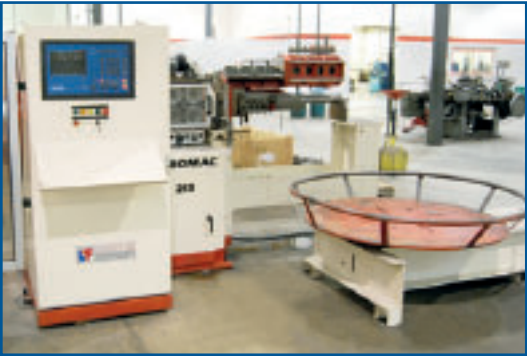
LATOIR ROBOMAC MODEL 213 3D CNC WIRE FORMING MACHINE
