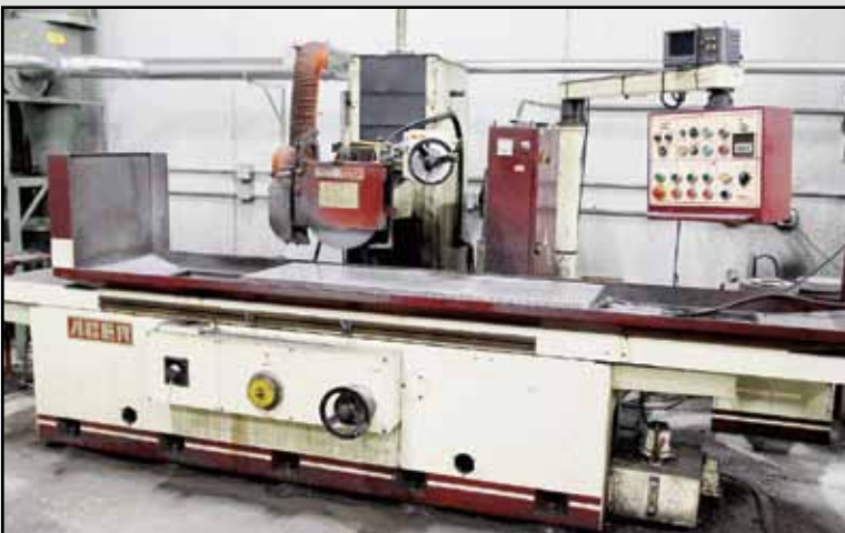
ACER AGS2060AHD Auto Horizontal Surface Grinder
