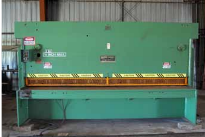
HTC 250-12A Hydro-Mechanical Shear, S/N. A172496; 12' x 1/4" Capacity, Power Back Gauge ▲
