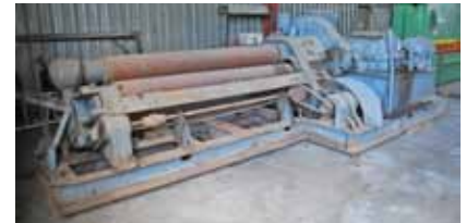
WEBB 9L 1308 Three-Roll Mechanical Plate Bending Roll, S/N. 6063; 8' 2" x 3/4" Capacity, 20 HP Motor ▲
